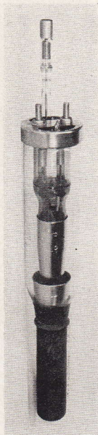
Vacuum Tube—10 Kw, Used in Trans- atlantic Telephony—1929
