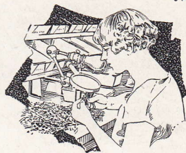
Inspecting Multiple Bank Springs
