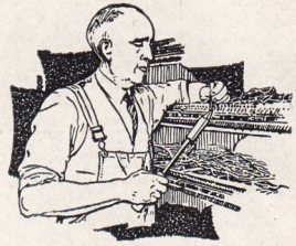
Soldering the Switchboard Connections
