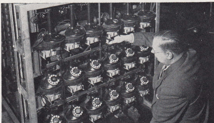
This Bell Laboratory Machine Automatically Tests the Life of the Switchhook Contacts on Eighteen Telephones Simultaneously
