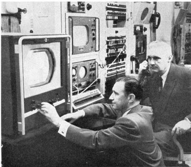
A Bell Laboratories and a Long Lines engineer check the quality of a full-color picture at a special monitoring position in one of the Bell System television network control centers.
