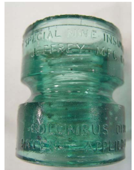
Right: This unusual insulator is marked "SPECIAL MINE INSULATOR, JEFFREY MFG CO on the top half and COLUMBUS OH, PAT APPLIED FOR on the bottom. The insulator is open on both ends and threaded all the way through. What's that all about?
