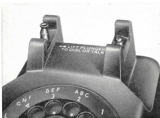
Fig. 3—500F Telephone Set Showing Plunger Switch and Instruction
