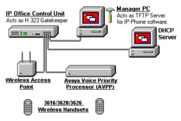
Use of the 3616, 3620 and 3626 phones via an AVPP is supported on the IP Office IP403, IP406 (V1 and V2) and IP412 units. The Small Office Edition unit is able to support a built-in wireless access point. However, this does not provide Quality of Service (QoS) support.
