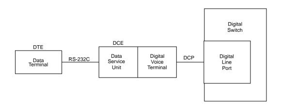
Figure 21-13. A Block Diagram of Z702AL1 Data Service Unit Interfaces
