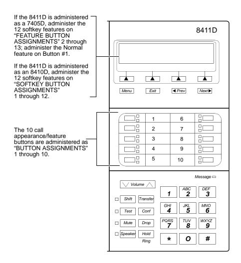
Figure 12-18. Button Numbering for Administering the 8411 Voice Terminal Connected to a System 75, a DEFINITY G1 or G3, or a DEFINITY ECS
