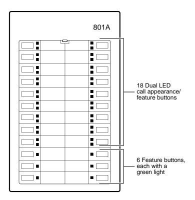
Figure 20-4. The 801A Expansion Module
