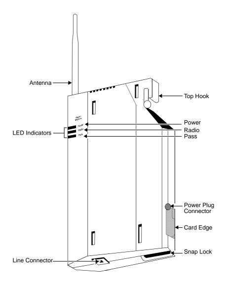
Figure 18-7. The MDW 9000 Telephone, Radio Module
