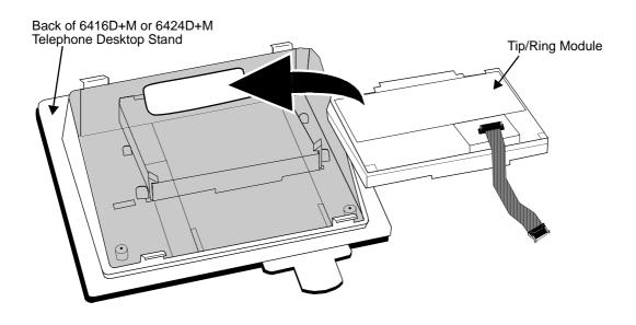
The 100ATip/Ring Module Being Installed in the Desktop Stand **Figure 20-8.** of a 6416D+ or 6424D+ Telephone
