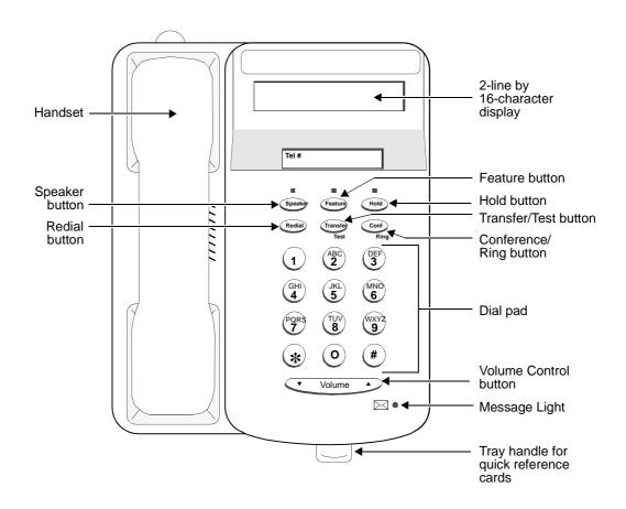
Figure 7-2. The 6402D Telephone
