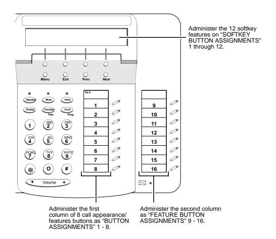
Button Numbering for Administering the CALLMASTER V Telephone Console Connected to a DEFINITY ECS Release 6.1 and Later **Figure 13-10.**
