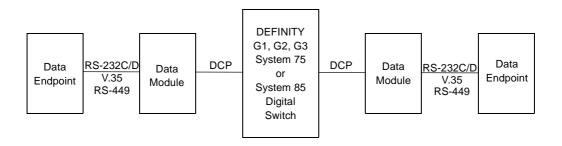
Figure 2-3. Data Link Components
