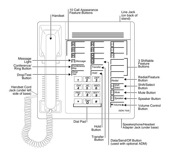
The 7505 Asynchronous Data Modular Terminal Figure 17-1.
