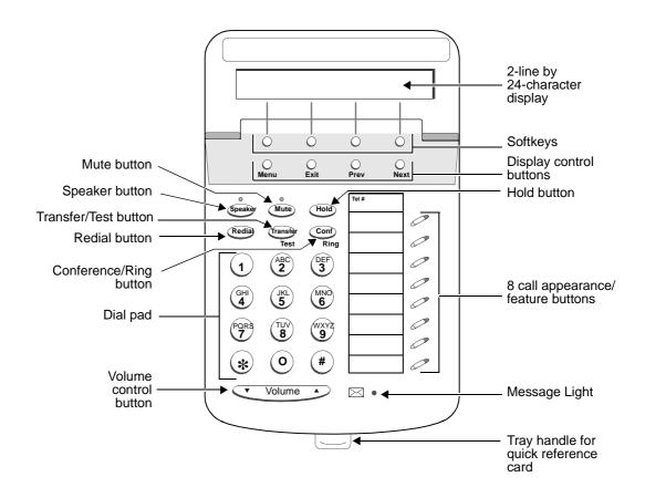
Figure 7-5. The 6408D+ Telephone (With Display)
