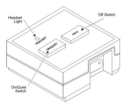
Figure 20-10. The 500A Headset Adapter
