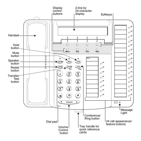
Figure 7-9. The 6424D+ and 6424D+M Telephone
