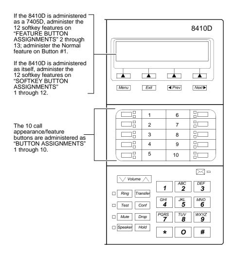
Figure 12-13. Button Numbering for Administering the 8410 Voice Terminal Connected to a System 75, a DEFINITY G1 or G3, or a DEFINITY ECS
