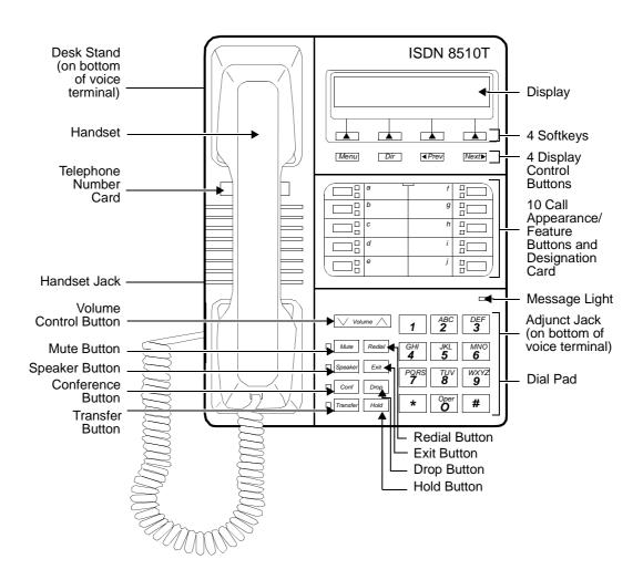
Figure 17-5. The ISDN 8510T Voice/Data Terminal
