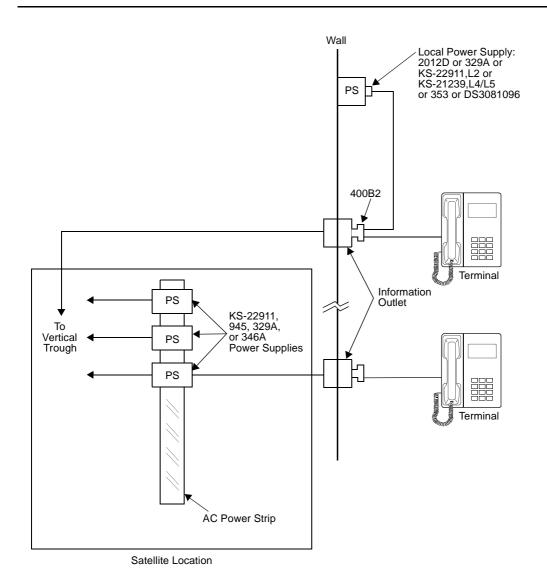
Figure 4-1. Local and Satellite Power Sources for Voice Terminals Adjuncts
