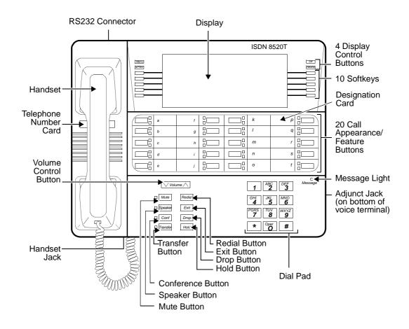
Figure 17-6. The ISDN 8520T Voice/Data Terminal
