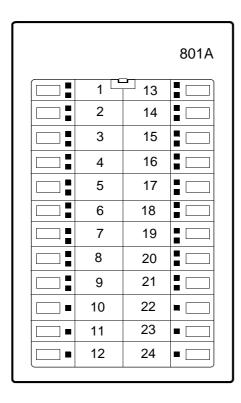
Figure 20-5. **Button Numbering for Administering the 801A Expansion Module**
