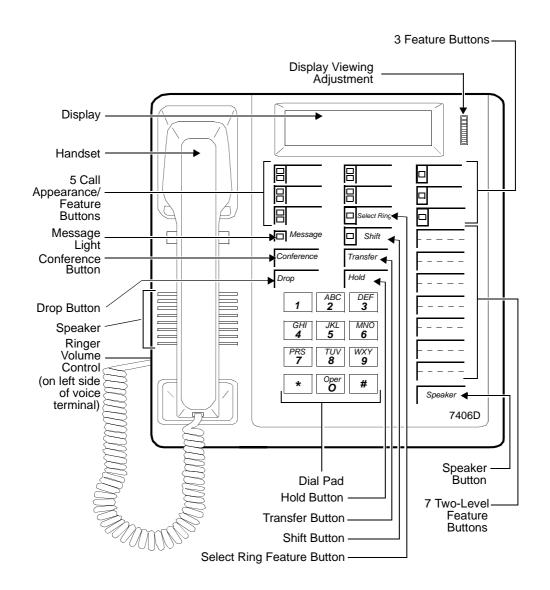
Figure 11-10. The 7406D (7406D01A or 7406D03A) Voice Terminal with Display
