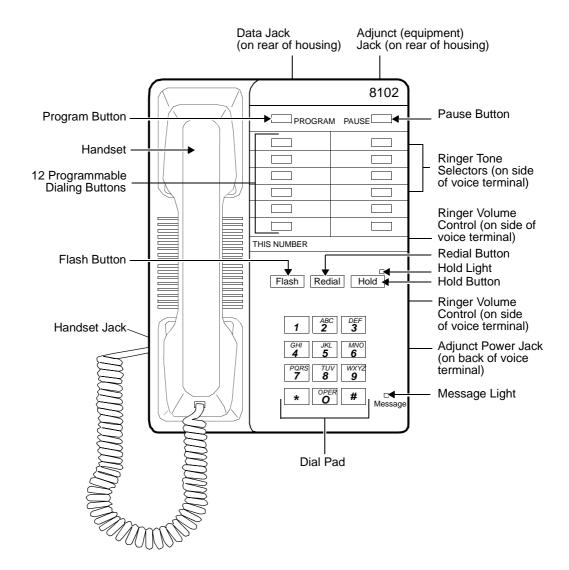
Figure 16-3. The 8102 and 8102M Telephone
