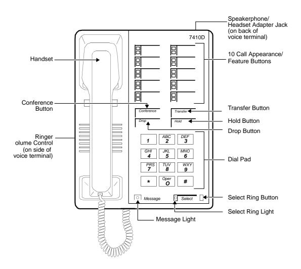
Figure 11-26. The 7410D (7401D01A) Voice Terminal
