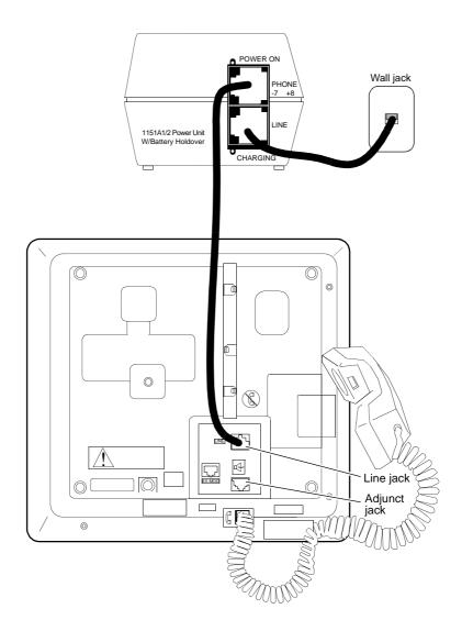
Figure 4-4. Local Powering Arrangement (Using the 1151A1/A2) for: ISDN-T Voice Terminals; the DCP 7444 and 8434/8434DX Voice Terminals (for their VF Displays); the 8411; any 8400 or 6400 Series Telephone with an Attached Expansion Module; and Adjuncts Connected to All Telephones Except the 8102
