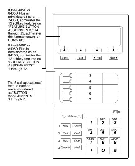
Figure 12-10. Button Numbering for Administering the 8405 Voice Terminal Connected to a System 85 or a DEFINITY G2
