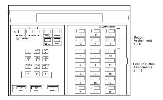
Figure 13-9. Button Numbering for Administering the CALLMASTER IV Voice Terminal Connected to a DEFINITY ECS G3V3 or Later
