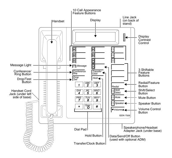
Figure 17-2. The 7506 Asynchronous Data Modular Display Terminal
