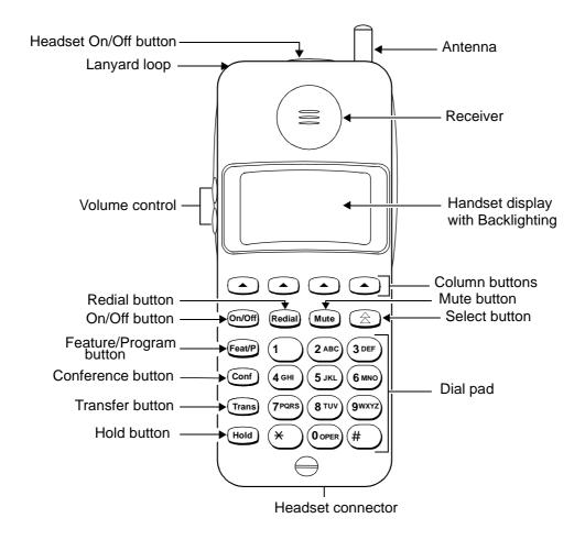
Figure 18-10. The MDW 9031DCP Wireless Pocket Phone
