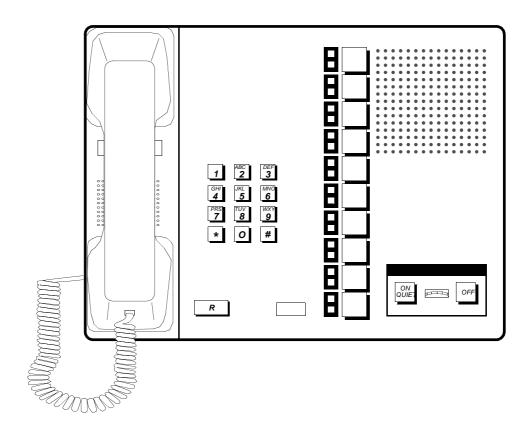
Figure 19-3. The 10-Button MET Set with Speakerphone
