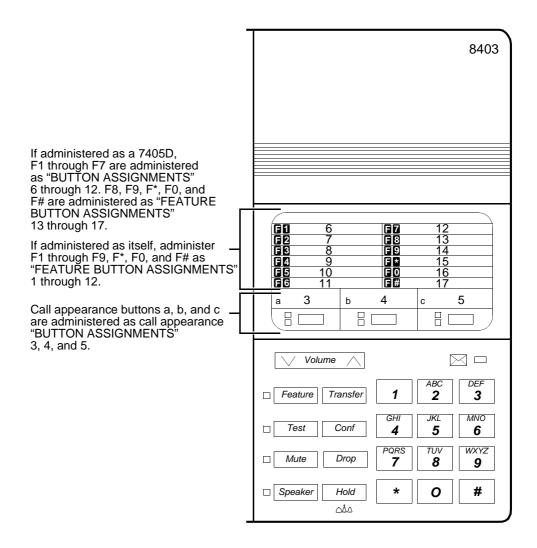
Figure 12-4. Button Numbering for Administering the 8403 Voice Terminal Connected to a System 85 or a DEFINITY G2
