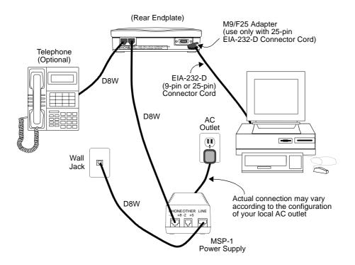
Typical Installation of the International Configuration, Including Telephone and Separate Power Supply **Figure 21-7.**
