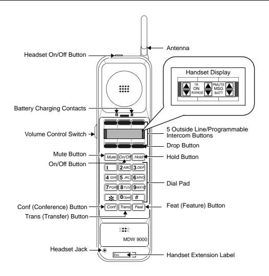
Figure 18-5. The MDW 9000 Telephone, Including Enlarged Display Area
