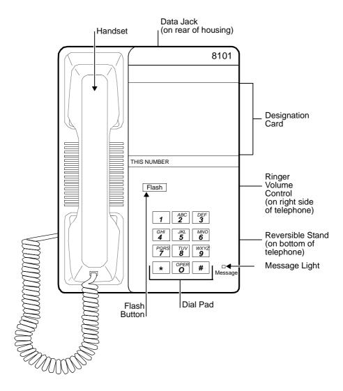
Figure 16-2. The 8101M Telephone
