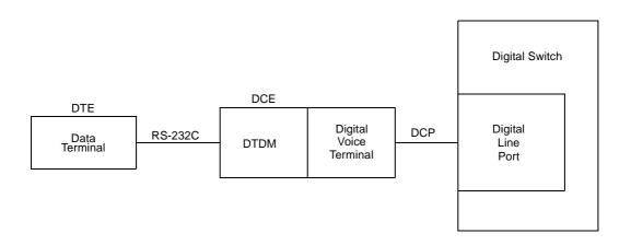
Figure 21-11. A Block Diagram of DTDM Interfaces
