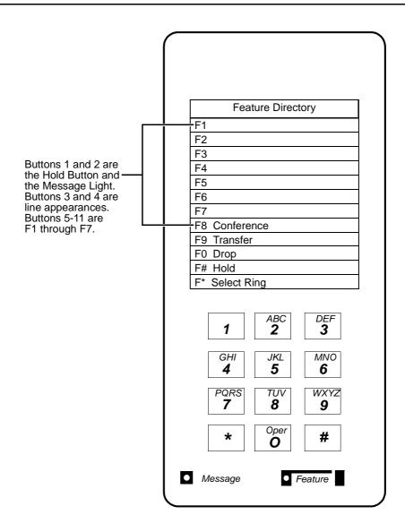
**Button Numbering for Administering the 7401D and 7401 Plus Voice Figure 11-3.** Terminals Connected to a System 85 or a DEFINITY G2
