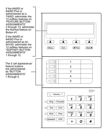
Figure 12-9. Button Numbering for Administering the 8405 Voice Terminal Connected to a System 75, a DEFINITY G1 or G3, or a DEFINITY ECS
