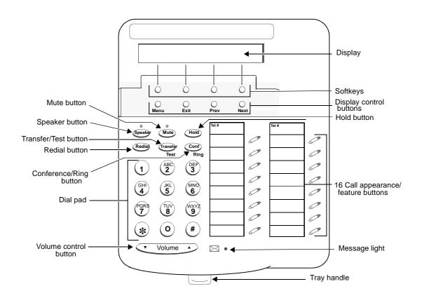
Figure 7-7. The 6416D+ and 6416D+M Telephone
