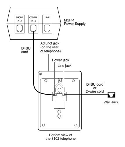
Figure 4-3. **Local Powering Arrangement (Using the MSP-1) for Adjuncts Connected to the 8102 Analog Telephone**
