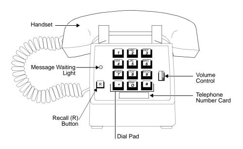
Figure 14-5. The 2500 DMGC Telephone
