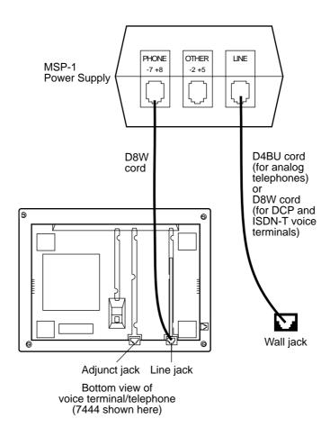
Figure 4-2. Local Powering Arrangement (Using the MSP-1) for: ISDN-T Voice Terminals; the DCP 7444 and 8434/8434DX Voice Terminals (for their VF Displays); and Adjuncts Connected to All Telephones Except the 8102
