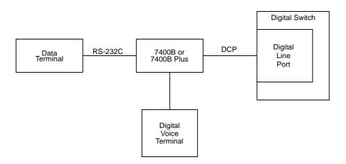
Figure 21-3. A Block Diagram of the 7400B Interface
