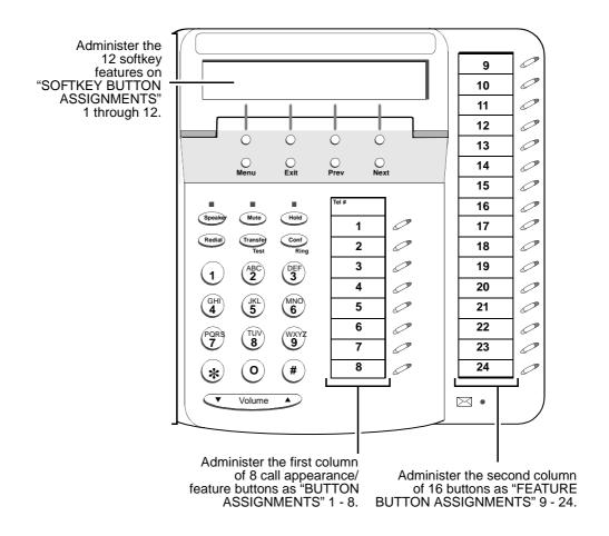
Button Numbering for Administering the 6424D+ or 6424D+M Telephone Figure 7-10. Connected to a DEFINITY System Release 6.1 or Later
