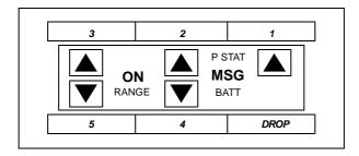
Figure 18-3. Button Numbering for a MDC 9000 Connected to System 75, a DEFINITY Generic 1 or Generic 3, or a DEFINITY ECS
