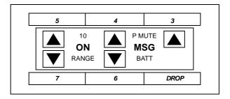
Button Numbering for an MDW 9000 Connected to a **Figure 18-9.** System 85 or a DEFINITY Generic 2
