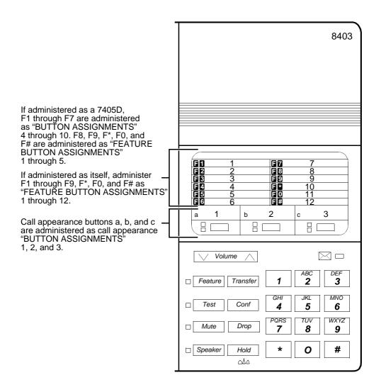
Figure 12-3. Button Numbering for Administering the 8403 Voice Terminal Connected to a System 75, DEFINITY G1 or G3, or DEFINITY ECS
