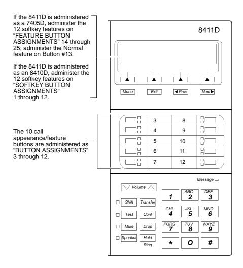
Figure 12-19. Button Numbering for Administering the 8411 Voice Terminal Connected to a System 85 or a DEFINITY G2
