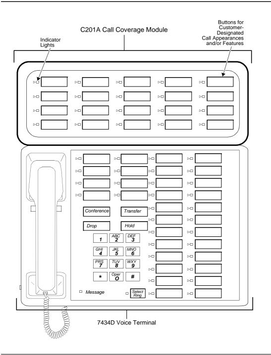
Figure 20-1. The C201A Call Coverage Module Mounted on a 7434D Voice Terminal
