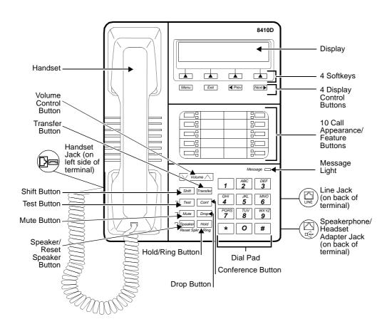
Figure 12-11. One Version of the 8410D Voice Terminal (with Display)
