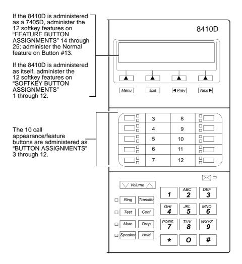
Figure 12-14. Button Numbering for Administering the 8410 Voice Terminal Connected to a System 85 or a DEFINITY G2
