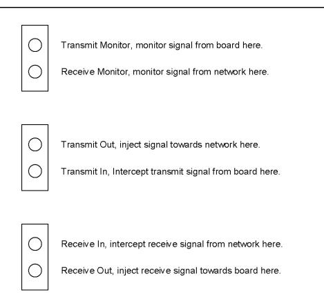
Figure 6-16. CSU Bantam Jacks. Ordering Is as They Appear on the Module Faceplate
