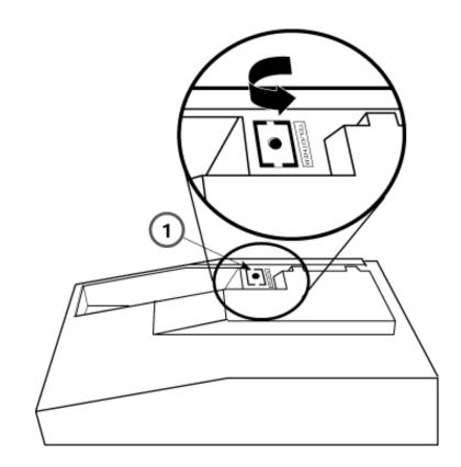
Figure 3-38. Removing the Jack Guard
