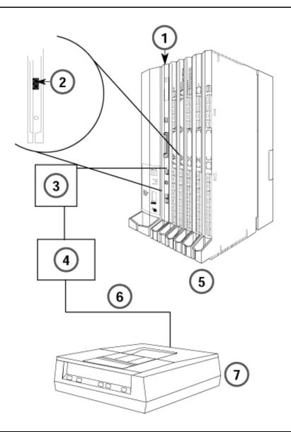
Figure 5-7. Connecting a Printer Within 50 ft. (15.2 m)
