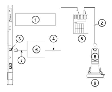
Figure 5-5. Connecting a CAT and Printer on the Same AC Outlet
