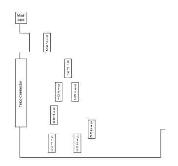
Figure 6-12. 100 DCD Data Port DIP Switch Placement
