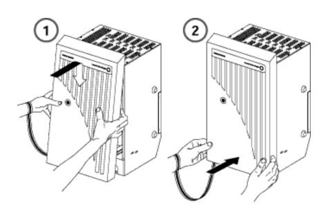
Figure 2-11. Installing the Cover for the Carrier
