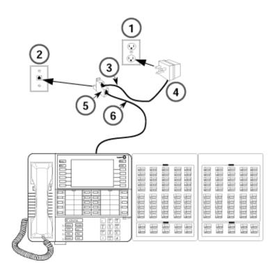
Figure 3-25. Wiring an MLX Telephone for Auxiliary Power
