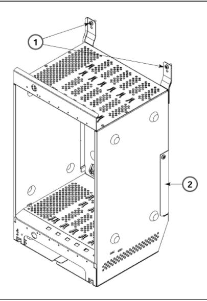
Figure 2-4. Securing the Left and Right Bracket
