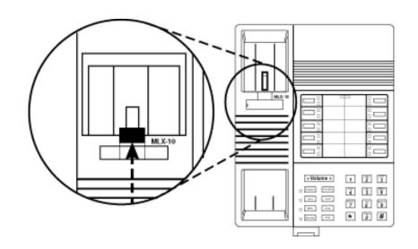
Figure 3-5. Removing the Handset Holder
