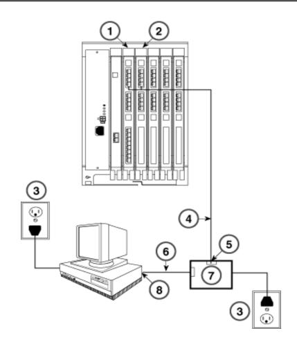
Figure 6-6. Single User Workstation with ISDN Router
