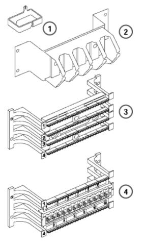
Figure 4-2. RJ21X Wiring Field Hardware
