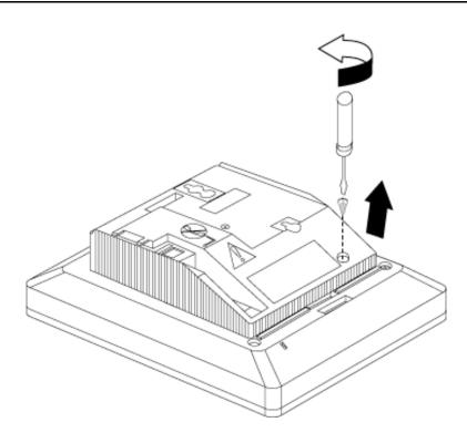
Figure 3-32. Releasing the Module Cover Screw
