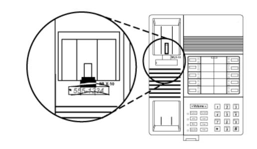
Figure 3-7. Replacing the Extension Label
