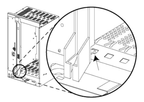
Figure 2-7. Installing the Processor into the Carrier
