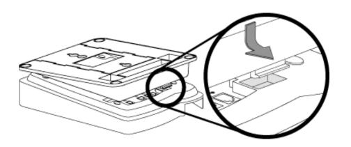
Figure 3-13. Attach Bottom of 4400-Series Telephones to Wall-Mounting Stand
