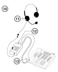
Figure 3-20. Manual and One-Touch Headset Operation
