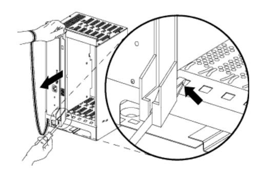
Figure 2-8. Removing a Module
