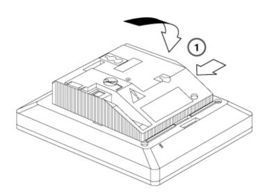
Figure 3-40. Lowering and Locking the Module Cover
