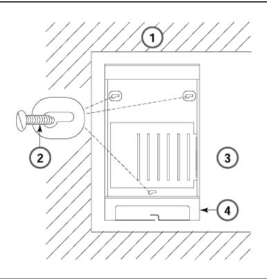
Figure 2-1. Marking the Basic Carrier Screw Holes
