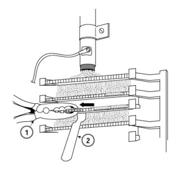
Figure 3-16. Removing the Connecting Block
