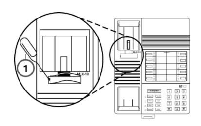
Figure 3-3. Removing the Extension Label
