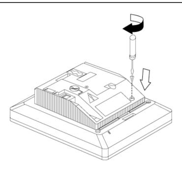
Figure 3-41. Replacing and Tightening the Module Cover Screw
