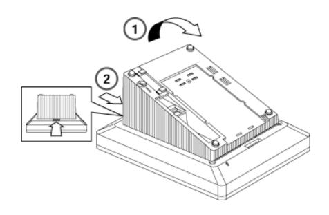
Figure 3-1. Adjusting or Removing the Desk Stand
