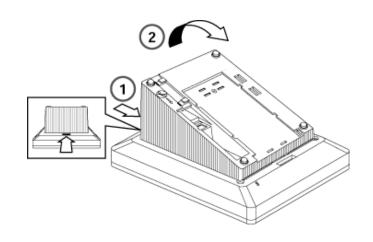
Figure 3-30. Releasing the Deskstand
