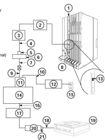
Figure 5-8. Connecting a Printer More Than 50 ft. (15.2 m) Away
