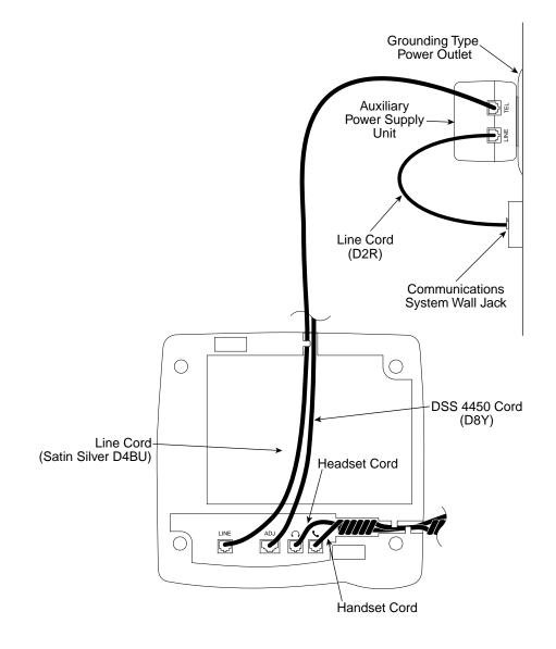
Figure 3-12. Jacks and Placement of Cords for the 4424LD+ and 4424D+ Telephones Including Auxiliary Power Supply Unit and DSS 4450
