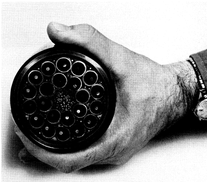
Cross-section view of the 22-tube coaxial cable, part of the L5 transmission system. This super-capacity transmission facility can carry 108,000 simultaneous telephone conversations—more than three times the capacity of previous cable systems.
