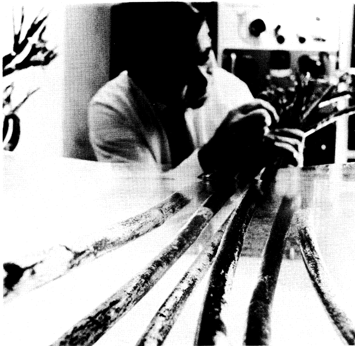
The long search for a "waterproof" cable neared its end in about 1966 when M. C. Biskeborn advocated a British concept of using a petroleum jelly blend to fill the air spaces inside a cable. Even with the outer sheath of such a cable perforated and the cable completely submerged in water, tests such as that being performed here by Ambrose Vallyely cannot detect any appreciable entrance of water.
