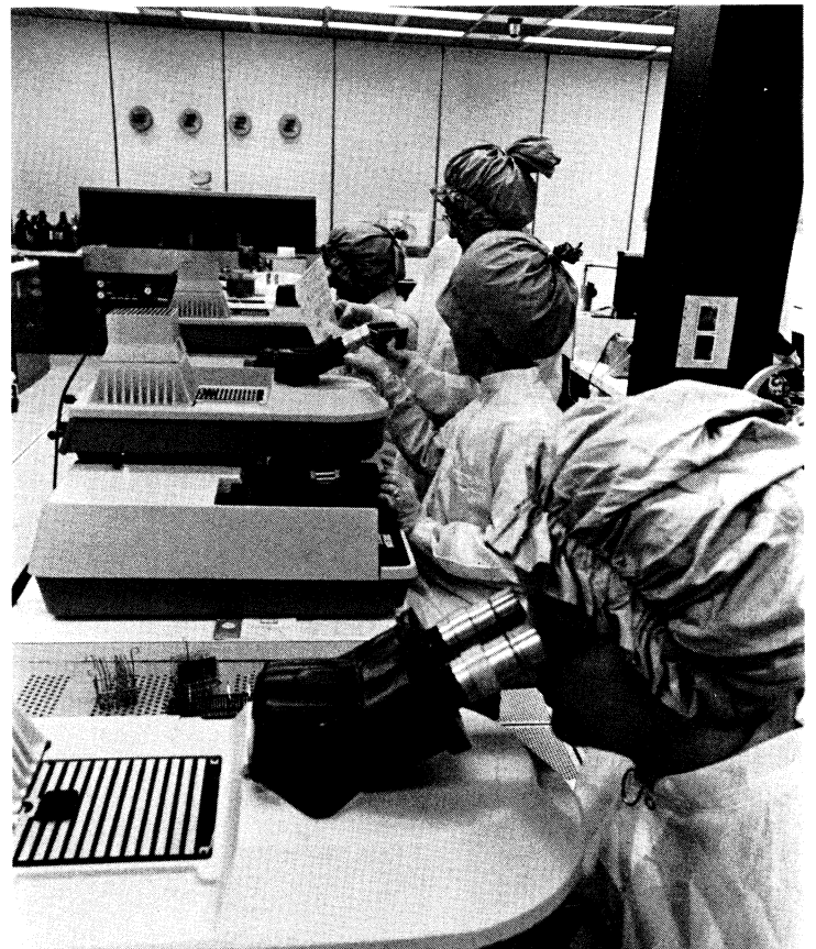
The manufacture and assembly of integrated circuits takes place today in ultra clean facilities such as this Design Development Laboratory (DDL) at Allentown, Pennsylvania. Bell Labs and Western Electric engineers share responsibility for technical supervision, while highly skilled personnel from Western Electric operate the facilities.
