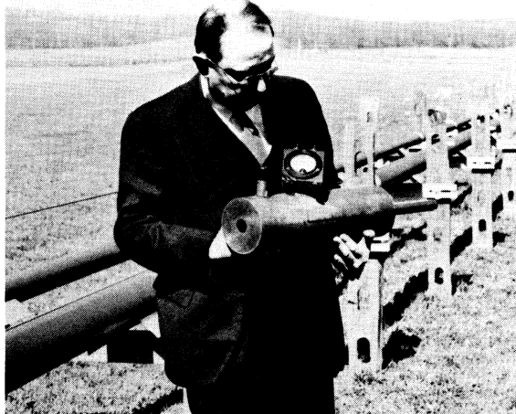
In this photo taken in 1936, G. C. Southworth holds one of the resonant chambers used for tests of waveguide transmission. Behind him are two experimental transmission lines.
