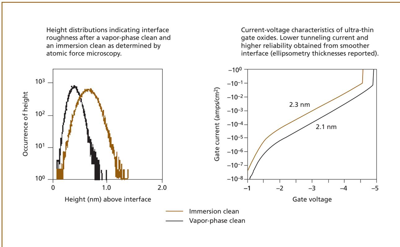
**Figure 5.** Graphs showing lower tunneling current resulting from a smoother Si/SiO<sub>2</sub> interface.<sup>12</sup>
