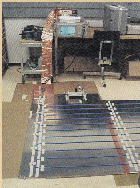
Figure 1. Cable layout on groundplane looking toward the ESD charging-end fixture
