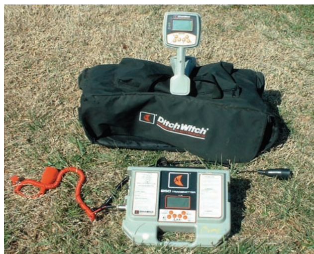
For toning, CommScope recommends equipment such as the DitchWitch 950R/T (shown above).
