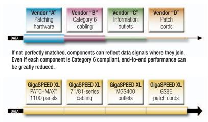
SYSTIMAX GigaSPEED XL components are precision engineered to provide a generous bandwidth margin that ensures absolute reliability through your entire channel.
