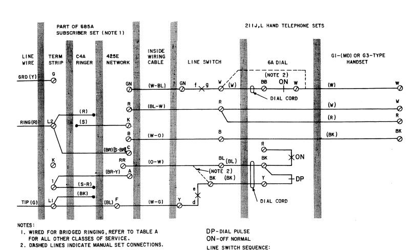
Fig. 1-\$211J/L Hand Telephone Set Connections Used With 685A Subscriber Set
