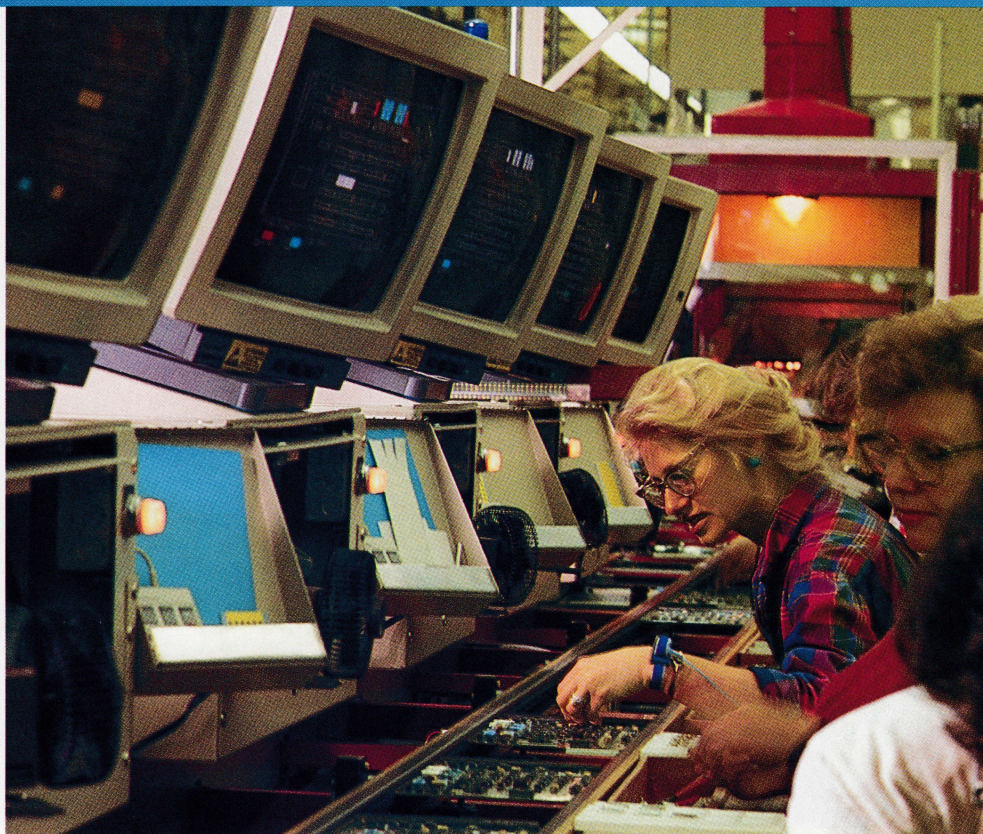
(Above) Workers at our Denver factory, with the push of a button, can bring circuit board assembly to a halt to trace and fix a problem.
