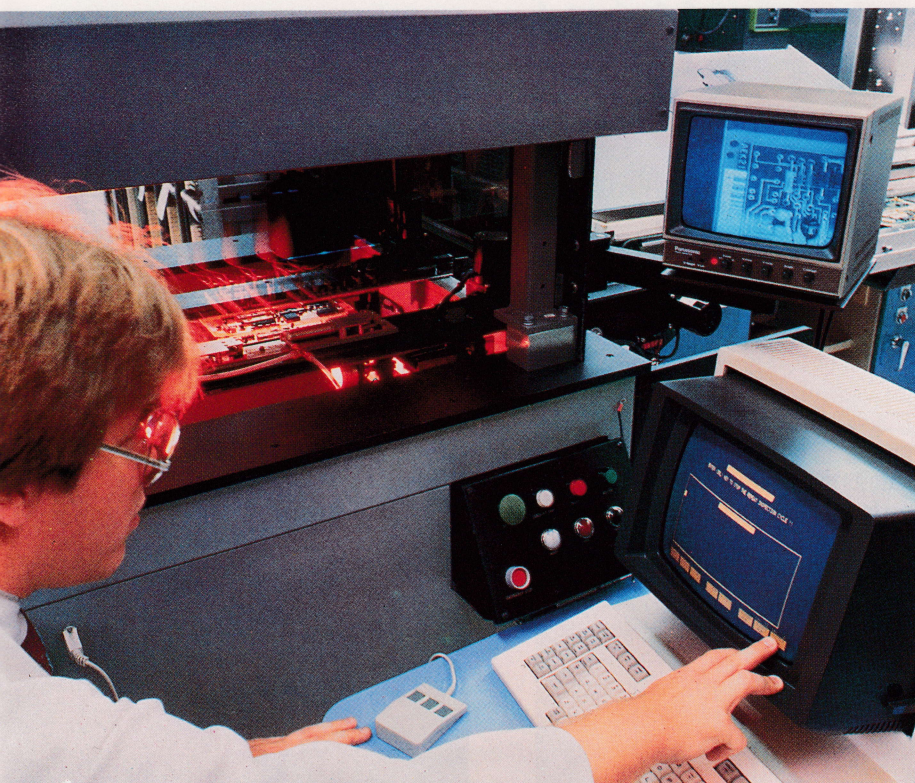
At left, Duncan Beech programs an inspection machine on a computerized circuit board manufacturing system.
