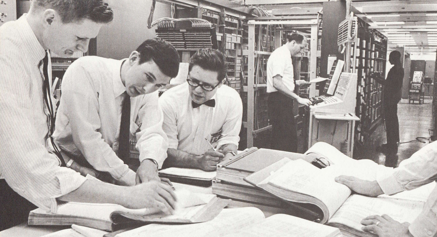
Bell Laboratories engineers at the new Indian Hill laboratory near Chicago test a "program" for an electronic switching system. Bays in the rear contain characteristic electronic switching equipment. These systems are somewhat like large computers but they must also meet many special requirements and there can be no "down time."
